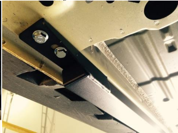
Figure 2: Passenger Side Jacking Rail
