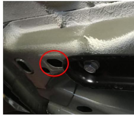
Figure 4: Slotted hole for offset stud
