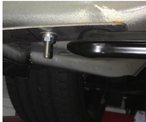
Figure 5: Steeda jacking rail front bracket
