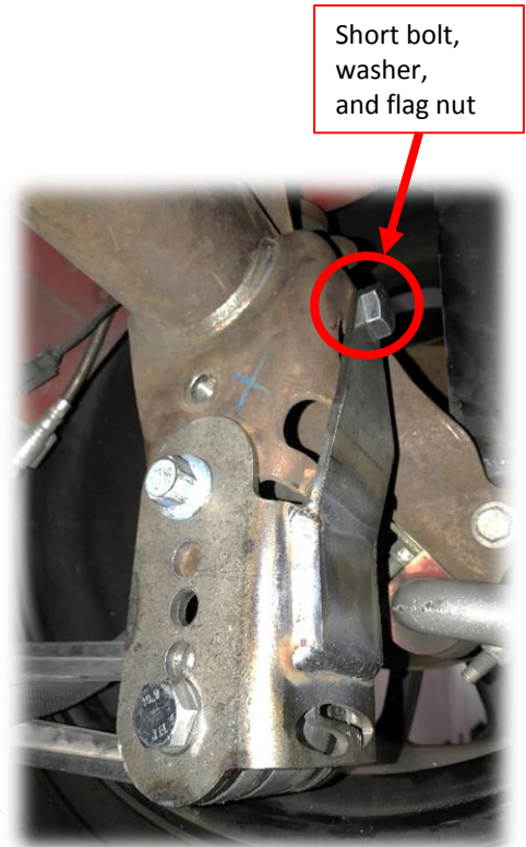
Figure 2: Passenger's side relocation bracket installed
