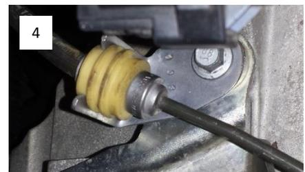
11. Remove the 3 bolts from the transmission cable bracket, and remove the bracket. **Note:** The longer bolt secures the clutch line bracket as well.
