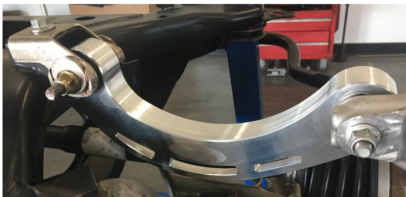
Figure 2: Steeda non-adjustable camber arm with the Steeda rear camber adjustment bracket (555-4126)
