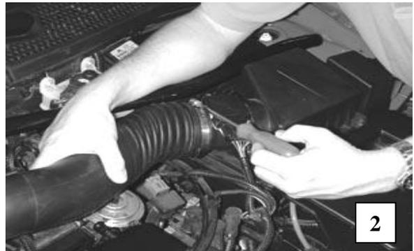
6. Disconnect the factory intake tube from the filter box. Loosen the hose clamp by the mass air meter and separate the tube from the air box. (Pic 2)
