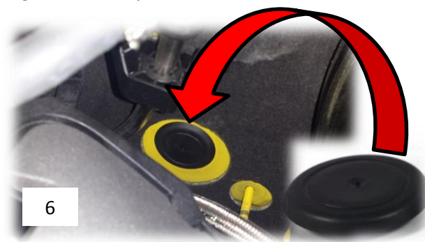
Figure 6: Sound tube plug installed
