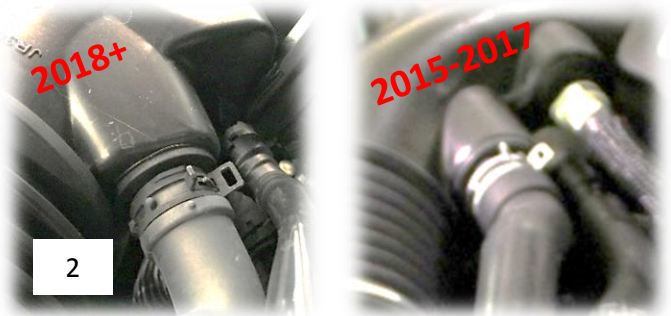
Figure 2: Hoses connected to factory intake tube
