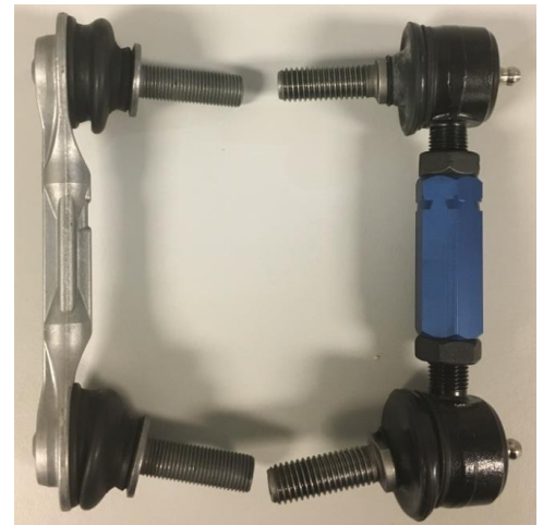
Figure 2: Factory vs Steeda rear swaybar endlinks
