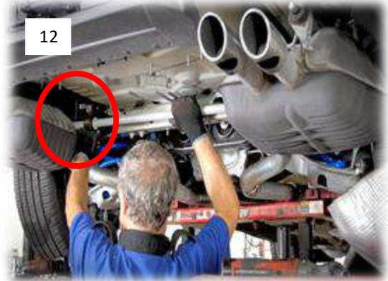
3. Install the swaybar endlinks and loosely tighten the nuts. Figure 13
