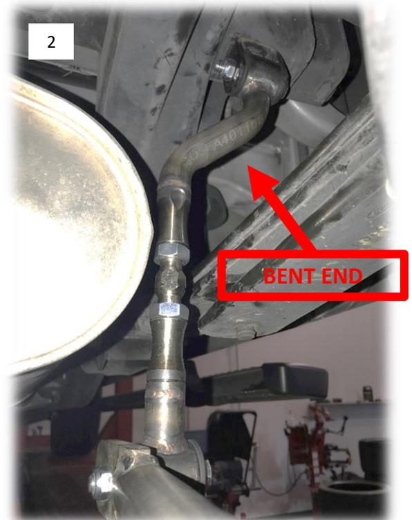
6. Loosely bolt the swaybar to the endlinks using a 17mm box end wrench, 17mm socket with a 3/8" ratchet, along with the provided 90mm long 10mm bolts, nuts, washers and **aluminum spacers which go between the bar and the endlink**.
