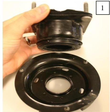
Separate the bearing and bushing from the spring seat itself with a screwdriver.
