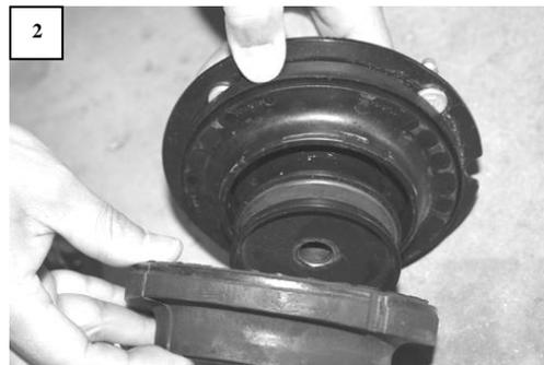
4. Remove the spring seat base from the new assembly. Insert the new spring base into the factory rubber spring seat. Be sure to keep the billet spring seat base face up to prevent disturbing the bearing inside. **Pics 3 & 4**
