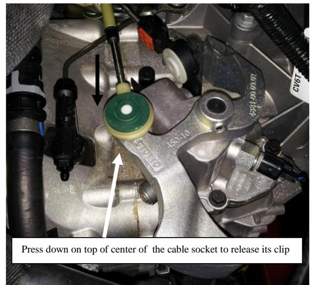
3. With the bracket assembly now exposed, shift the transmission input bracket so that the shifter cable socket is easiest to access. This can be done by turning the bracket by hand. See figure 2.
