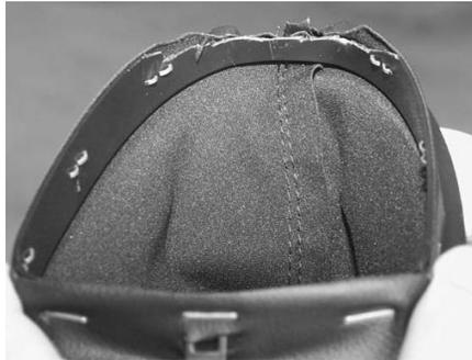
17. Install the shifter boot onto the lever.
