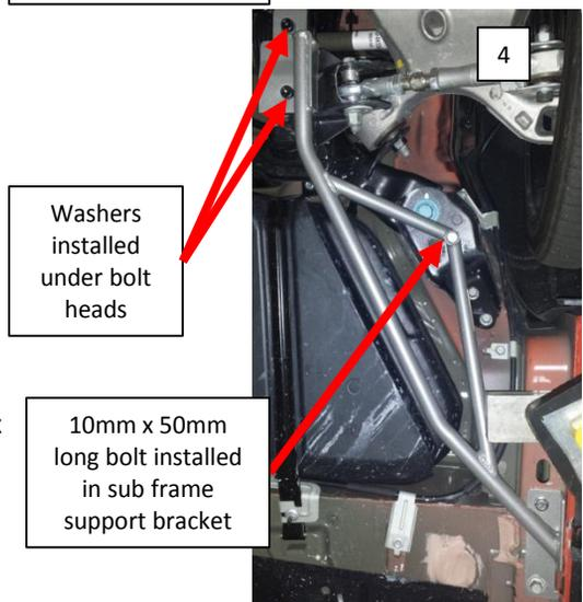
Washers installed under bolt heads
