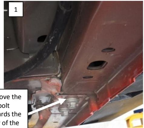
Remove the bolt towards the rear of the car
