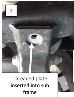
Threaded plate inserted into sub frame
