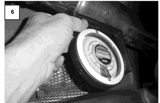
10. Adjust the new upper trailing arm center sleeve to lengthen or shorten the arm as necessary to correct the pinion angle. **One degree of pinion angle change is achieved by rotating the sleeve 1.65 turns.** Once you have achieved the desired pinion angle tighten the jam nuts securely against the adjusting sleeve. Thread lock is highly recommended.
