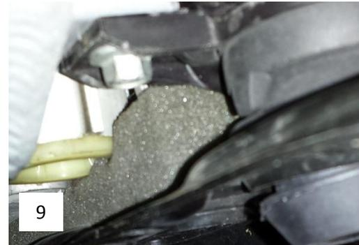
22. Gently pull the lower portion of the intercooler towards the front of the car and down to remove the intercooler.
