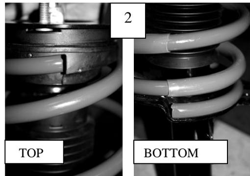
4. Re-attach the upper strut mount back to the car with the 4 nuts on top of the strut tower. The half moon notch should face the outside the vehicle. **Use Lock-Tight when reinstalling the swaybar endlinks.**
