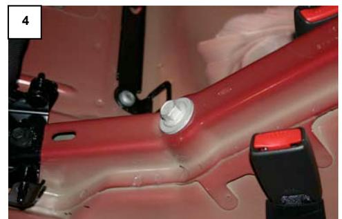
6. Tighten the trailing arm mounting bolts and the bracket bolts. Then, torque to factory specs. (129 ft/lbs.) Use the new supplied 14mm nut, bolt and washer on the chassis end.
