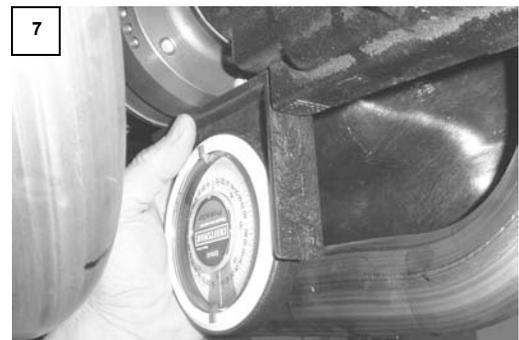
11. Re-measure the net pinion angle to insure you have achieved your desired setting and adjust if necessary.
