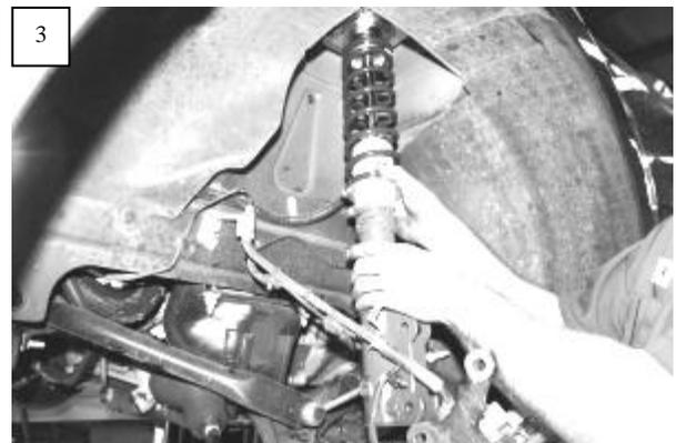
Carefully release the stock spring and remove the OE bump stop from the shaft of the strut.
