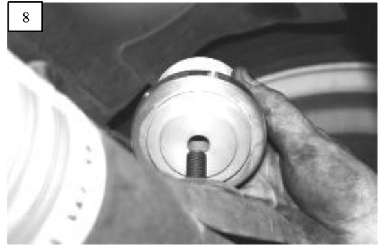
14. Reuse the upper rubber spring seat and the new Steeda lower spring seat, to secure the new Steeda spring in position.
