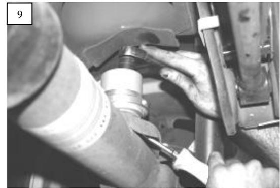
16. Install the new rear D-Spec shocks. From underneath the car have someone place the D-spec shock into position as you secure the upper nut.
