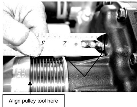
2. Pre-fit the pulley installer to the supercharger before proceeding to the next step. This will save time and allow the immediate installation of the new pulley.
